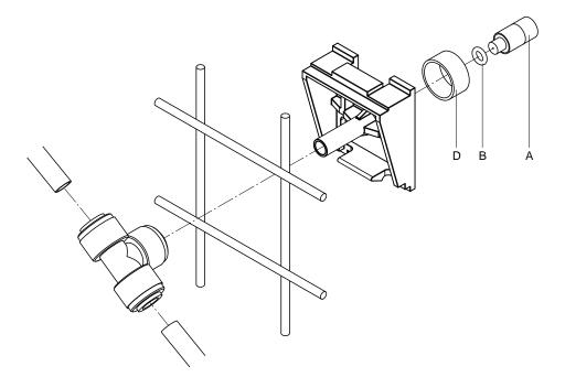
Abb. 12: Removal and installation of the nozzle holder
