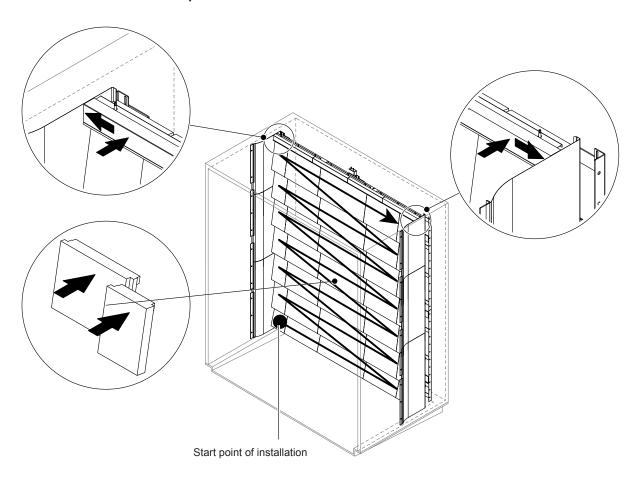
Abb. 10: Installation of the ceramic plates
