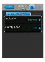
Indication: With this setting you determine whether maintenance messages ("Service") only or all Warning messages ("Warning") are outputted via the service relay of the remote operating and fault indication board.
