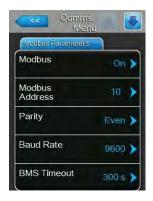
**Modbus**: With this setting you can activate ("On") or deactivate ("Off") communication via a Modbus network.
