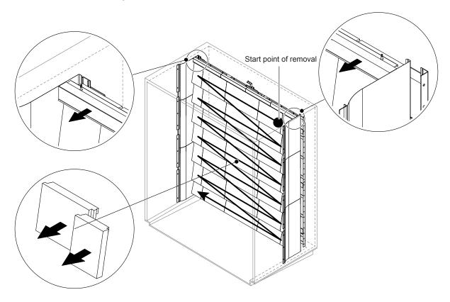
Abb. 9: Removal of the ceramic plates
