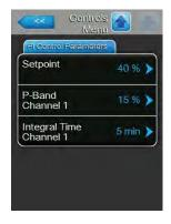
**Setpoint**: with this setting you set the humidity setpoint for the internal P/ PI controller in %rh.
