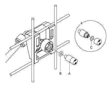
Abb. 11: Removal and installation of the spray nozzles
