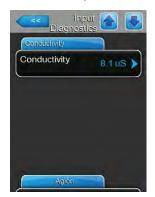
**Conductivity**: Actual conductivity of the supply water in  $\mu$ S.
