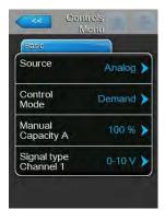
Source: with this setting you determine whether the control signal comes from an analogue source (signal of a humidity sensor or demand signal from an external humidity controller) or via Modbus.
